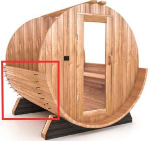
**Step 16** Screw the Bench Leg to the center of the Bench.
