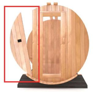
**Step 11** Fasten both segments to the middle section of the back wall. You'll need two 2 ½" screws.
