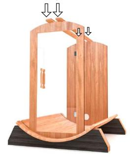
Place the Back Right Panel on the right side of the Central Back Panel. Slowly and carefully, lean the panel (diagonally) and insert it starting from the bottom. Work your way up the groove until both sides are connected. Make sure the bench brackets are facing the inside of the sauna.
