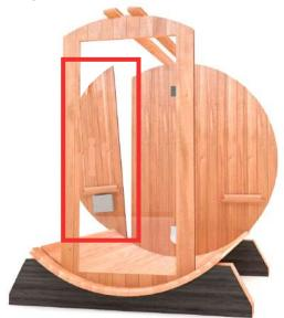
Step 8 Fasten both segments to the middle section of the back wall. You'll need two 2  $\frac{1}{2}$ " screws.
