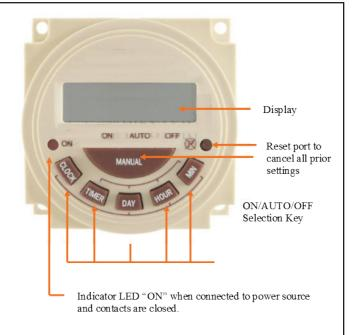
Press the **HOUR** key and then the **MINUTE** key to select the desired first ON time.
